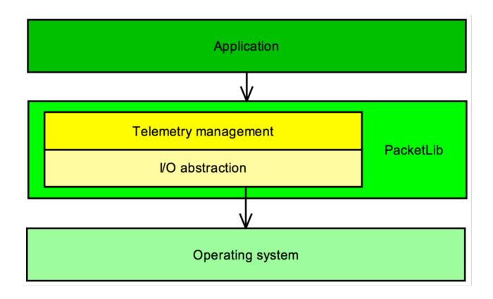
Figure 3.1: PacketLib layers
